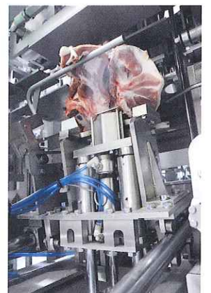
Automated arm-shoulder deboning robot
