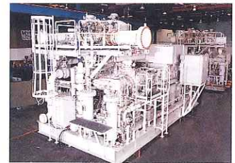
Hydrocarbon vapor recovery compressor package for sea-based platform
